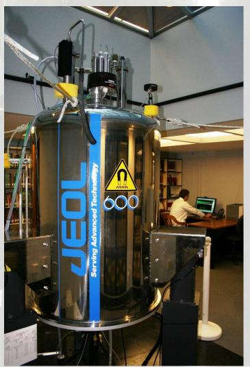
Instrument: JEOL ECA-600 MHz instrument
